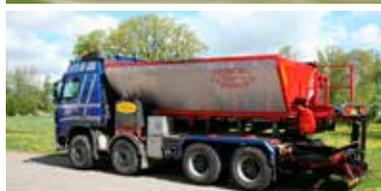
SG-series are linkage mounted and trailed sand- and salt spreaders, with a working width from 2 - 10 m. 100% hydraulic driven, the spreader has a positive feed floorbelt and 2 spread discs for a precise and accurate spread result.
