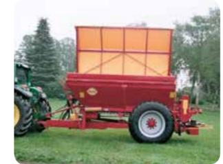
All BREDAL spreaders are fitted with a roller cover. Models K65, K85, K105 and K135 can also be fitted with a hydraulic cover.
