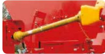
The wheel drive is connected to the conveyor belt gear by a PTO (power take-off) shaft. The standard 2-speed gearbox means that the rear hatch opening is always the right size for the material being spread. A gear for spreading particularly small amounts, ranging from 50 to 60 kg/ha, is available as an optional extra.
