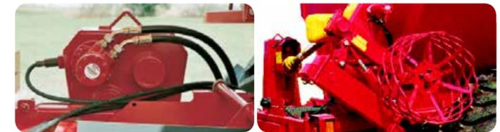
For electrical/hydraulic operation, the belt is controlled via a valve and oil motor. This facilitates spreading of large or small amounts. If required, the spreading wheel can remain in the machine as a backup, for example, if it becomes necessary to use a tractor that does not have a computer installed.
