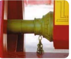
When using a 540 to 1,000 gear or 1,000 to 540 gear, it is possible to use tractors that cannot operate at both PTO speeds.
