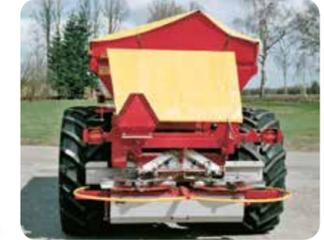
A roller cover for the conveyor belt and the spreading disc feed offers protection against the weather and against clumps of earth from the wheels.
