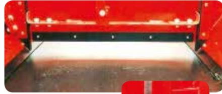
The rear hatch is fed by plastic guides, which ensures that the rear hatch will work even if the spreader is fully loaded. A hydraulic rear hatch is also available.
