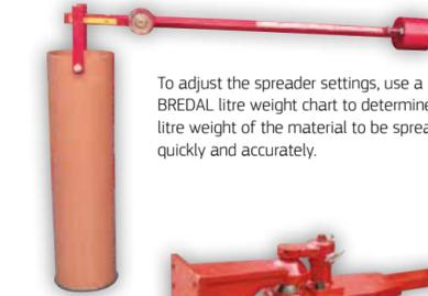
To adjust the spreader settings, use a BREDAL litre weight chart to determine the litre weight of the material to be spread quickly and accurately.
