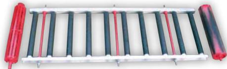
The conveyor belt rests on a powerful carrying frame with stainless steel beds and plastic-coated belt rollers with stainless steel shafts. The rollers have nylon, maintenance-free bearings. A close seal between bearing and roller prevents dust and foreign objects getting into the bearings.
