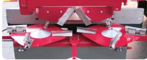
For spreading compost, sand and heavy materials, the direction of rotation (off centre) of the spreader discs can be changed. This feature is available in two ways on the SPC4500-1 and 2 spreading boxes.
