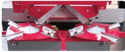
The standard SPC spreader system is fitted with spreader discs for spreading fertilizer up to 24 m and lime up to 16 m. Direction of rotation is centre line.
