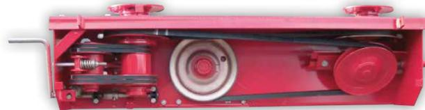
SPC4500-1 spreader system with headland gear.
