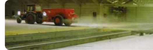
BREDAL spreaders work according to the double-overlap principle, i.e. at a spreading width of 12 m, the actual spread is 24 m. This principle ensures correct spreading.
