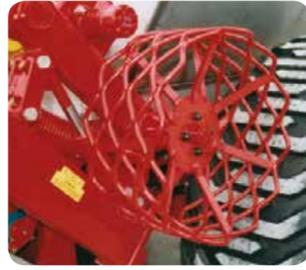
The mechanical drive wheel transfers the vehicle's speed, enabling the application rate to be adjusted according to the forward speed. The drive wheel is simply and robustly built and can be adjusted to suit different treads and wheel sizes. The drive wheel has a spring pressure of 400 kg. This guarantees that the vehicle wheel speed is always transferred accurately to the conveyor belt.
